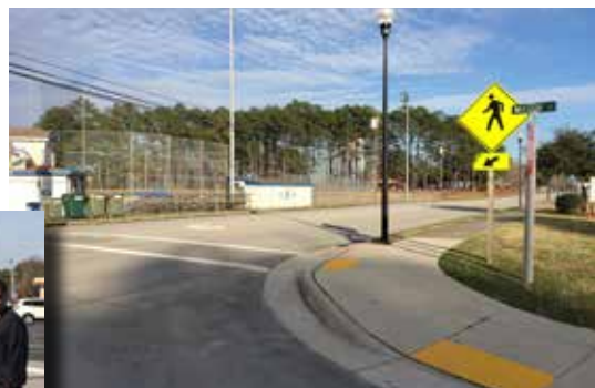
Left: Example of a missing curb ramp, at the crosswalk across Chatham Street at Haskett Street.
